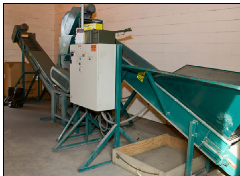
Fort Indiantown Gap purchased this brass crusher so expended brass casings could be recycled. In 2013, 94,000 pounds of expended brass casings were recycled. In 2014 the installation generated more than $280,000 in revenue from the entire Qualified Recycling Program. (Courtesy photo)
