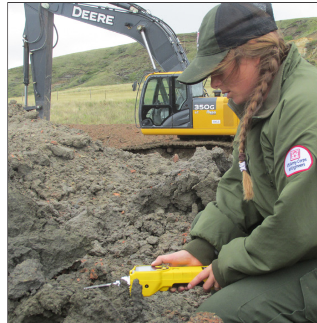
Garrison Project Office staff completed final reclamation of multiple oil well locations on the south shore of Lake Sakakawea in North Dakota. Hundreds of tons of soil had been excavated to meet USACE standards. (Photo courtesy of Army Corps of Engineers) RIGHT: Hattie Payne, natural resource specialist, tests soil for petroleum contamination, using a photoionization detector or PID gas meter on the oil well site in the Charlson Oil Field in McKenzie County, North Dakota. (Photo courtesy of Doug Hanson, Petro-Hunt)
