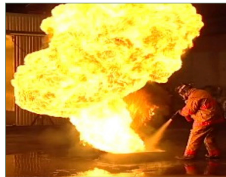
ABOVE: The U.S. Army Test and Evaluation Command performed hundreds of pan-fire tests during the developmental phase of the program. More pan-fire tests will be performed on the first non-ozone depleting substance hand-held fire extinguishers produced, prior to fielding. Performance qualification is required by the procurement contract. RIGHT: A Soldier outfitted in the fire resistant environmental ensemble, heavy flight gloves and other flight gear demonstrates a successful discharge operation and function of the non-ozone depleting substance hand-held fire extinguisher. (Courtesy photos)
