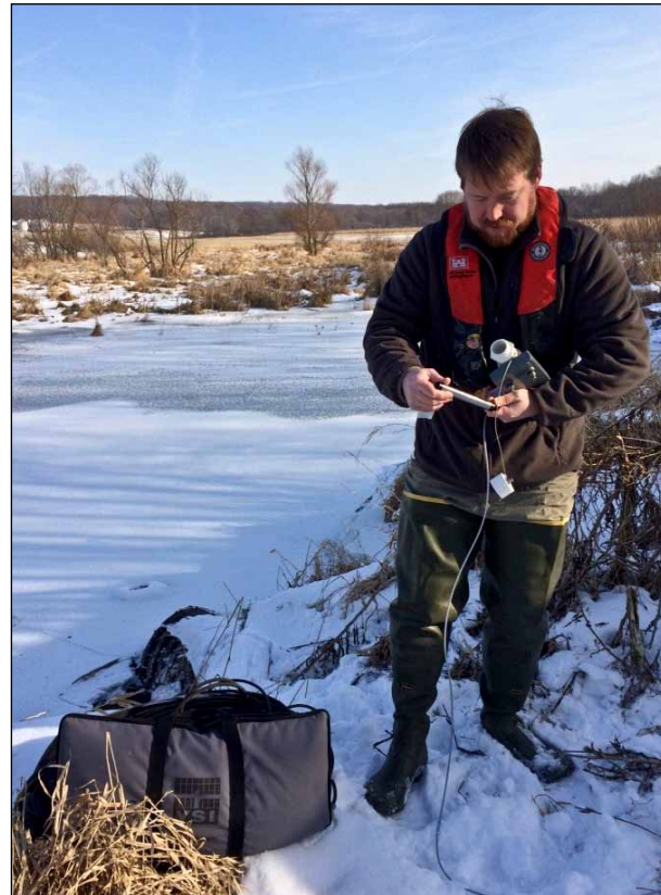
Carl Nim, Pittsburgh District biologist, deploys the data logger into the stream to test the water quality at Shenango River Lake downstream of a proposed well site. (Photo by Christina Barker)
