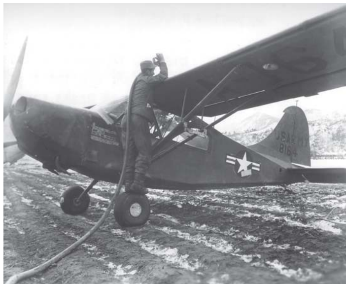
An aircraft mechanic refuels an L-5E observation aircraft RG 111, SC-356532
