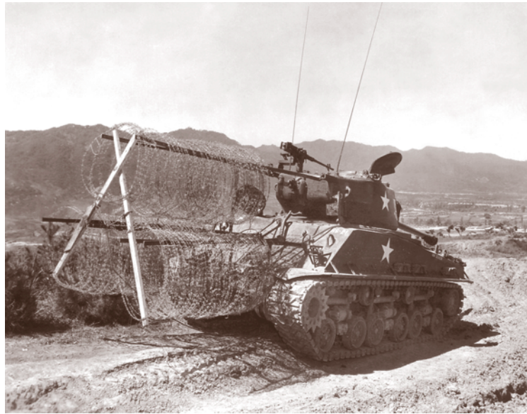
The 120th Combat Battalion experiments with a new method for replacing barbed wire while under fire RG 111, SC-410975
