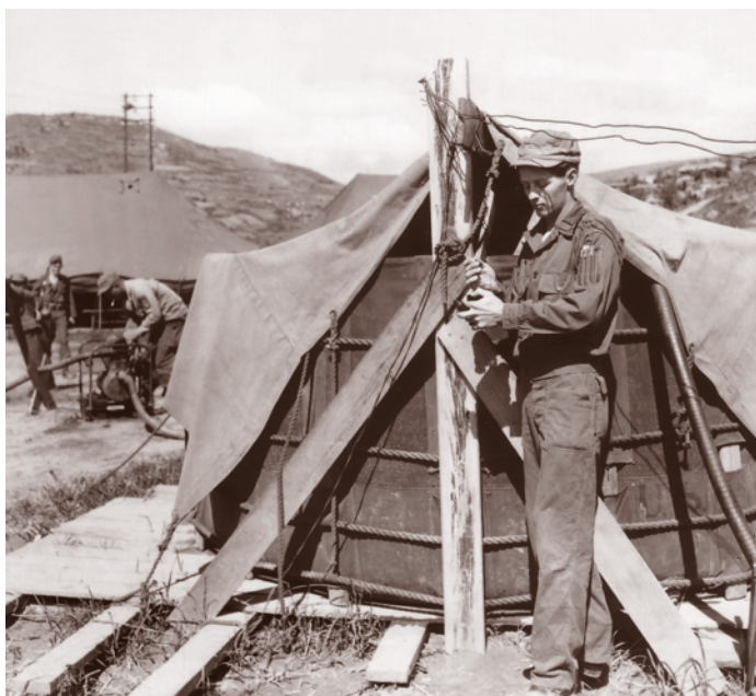
Pfc. Gene Davidson, a member of the water purification section, 453d Engineer Construction Battalion, tests the chlorine level in the water supply RG 111, SC-371535
