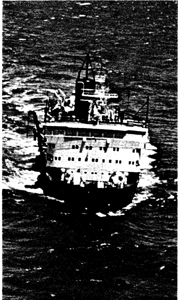
Hopper dredges can dump into open ocean water, but cost of long-haul disposal increases in direct proportion to distance from dredging site.
