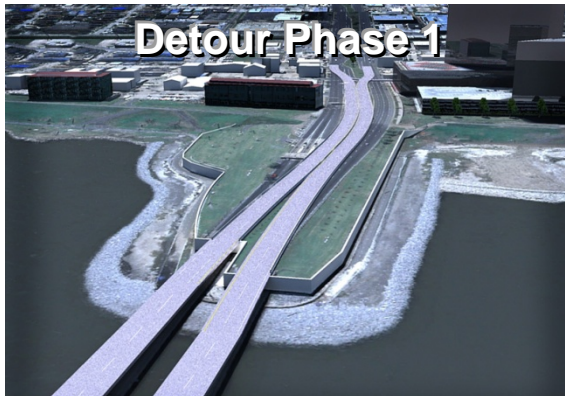
In the first phase of construction, the Causeway travel lanes were detoured into the median.
