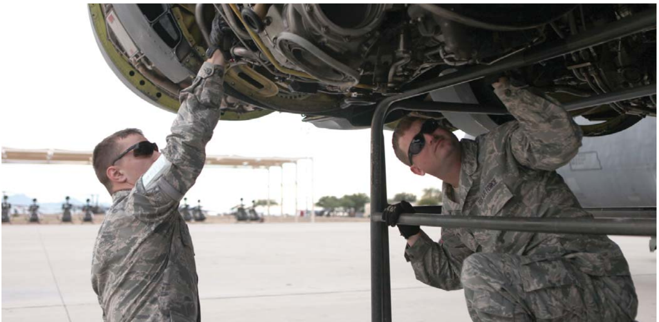
SrA Cody Grauel, Air Force Global Strike Command's 2nd Maintenance Squadron, left, inspects the No. 3 engine fuel pump on B-52H serial number 61-0007, the Ghost Rider, while SSgt Bradley Austin, with the Air Force Reserve Command's 307th Maintenance Squadron, inspects the No. 3 engine hydraulic pump. Tinker's B-52 System Program Office is one part of a team of units working together to get the B-52 back in flying condition to rejoin the Air Force fleet. (US Air Force photo by Teresa Pittman, AMARG)
