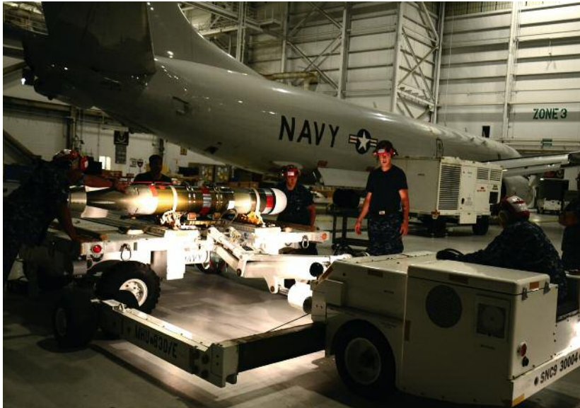
Aviation Ordnancemen assigned to Patrol Squadron (VP) 16, prepare to load a MK-54 torpedo onto a P-8A Poseidon aircraft in Jacksonville, Florida. PMA-290 testing activities involve the use of underwater sound/explosives in the marine environment, including systems under development. Eric A. Pastor
