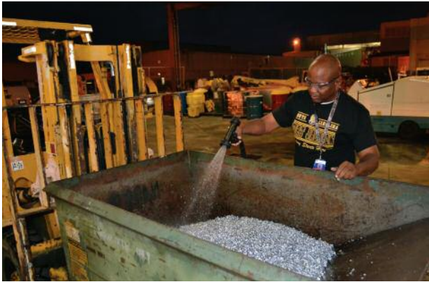
Charles Miller, an FRCSE material identifier, washes a bin of aluminum scraps collected through the manufacturing process. Washing the scraps removes oil residue and dust so the metal can be taken to Defense Logistics Agency Disposition Services for resale.
