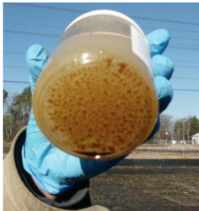
Dense non-aqueous phase liquid (DNAPL) was discovered as wells were being installed for substrate injection to address contamination in the shallow aquifer groundwater. The team developed an approach to remove the DNAPL, resulting in immediate contaminant mass reduction.
