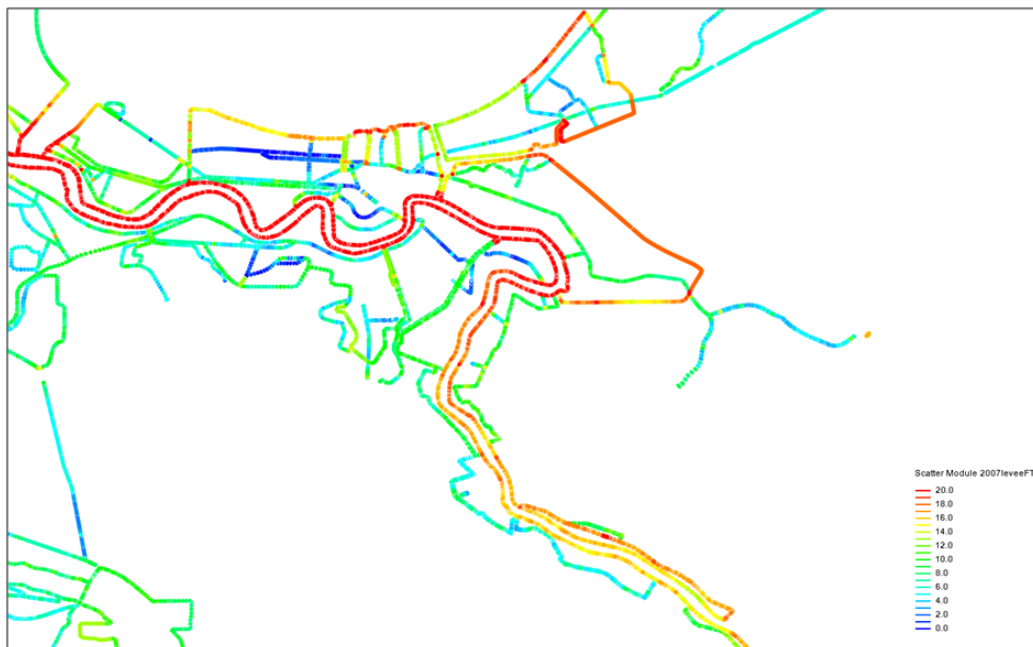
Figure 6.8. Elevations of levees, road systems and other structures represented as sub-grid scale features in the Without HSDRRS condition ADCIRC grid.
