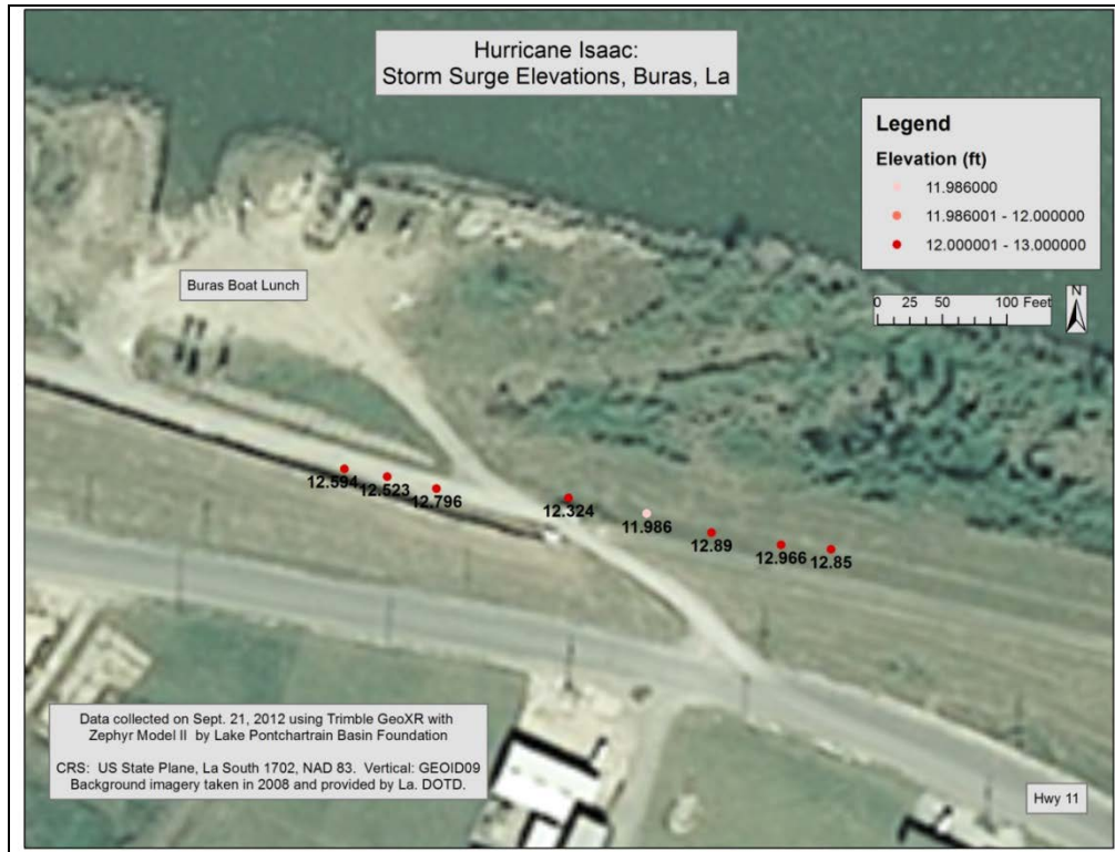
Figure 4.18 Recorded high water marks on the west bank Mississippi River Levee near Buras courtesy of the Lake Pontchartrain Basin Foundation.
