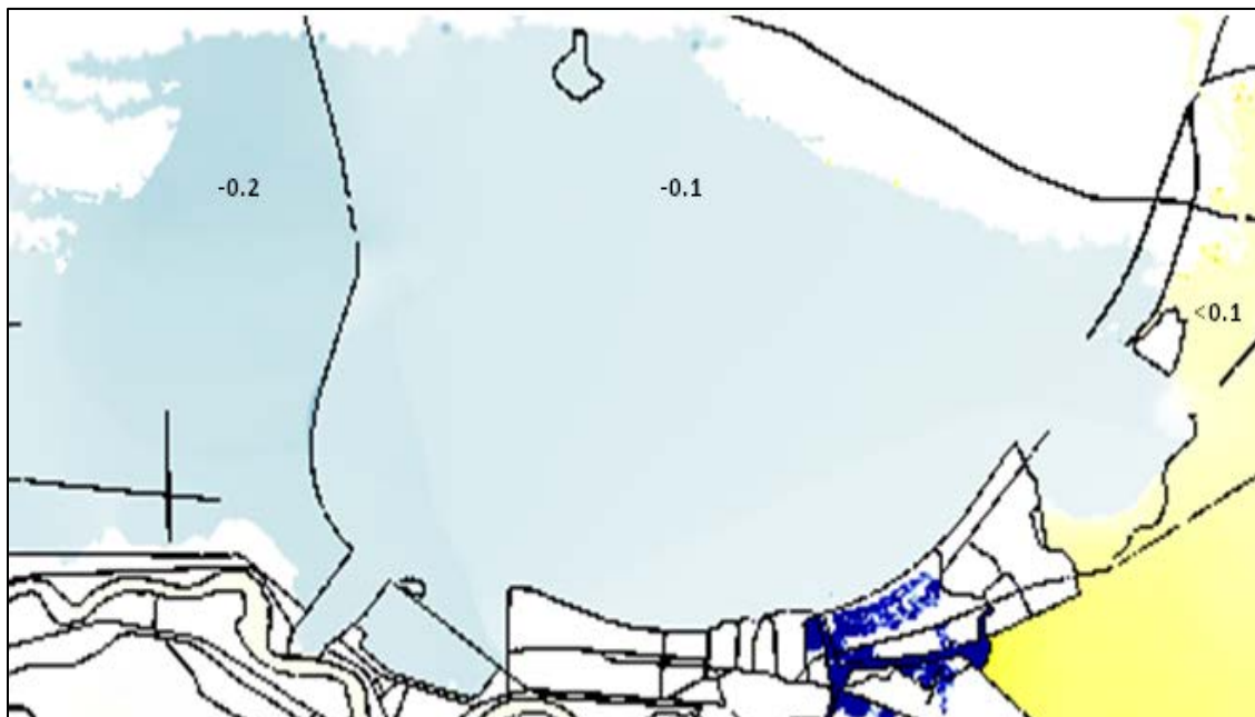
Figure 7.2.1 Difference in ADCIRC predicted peak water level for Hurricane Isaac in St. Tammany and Tangipahoa Parishes
