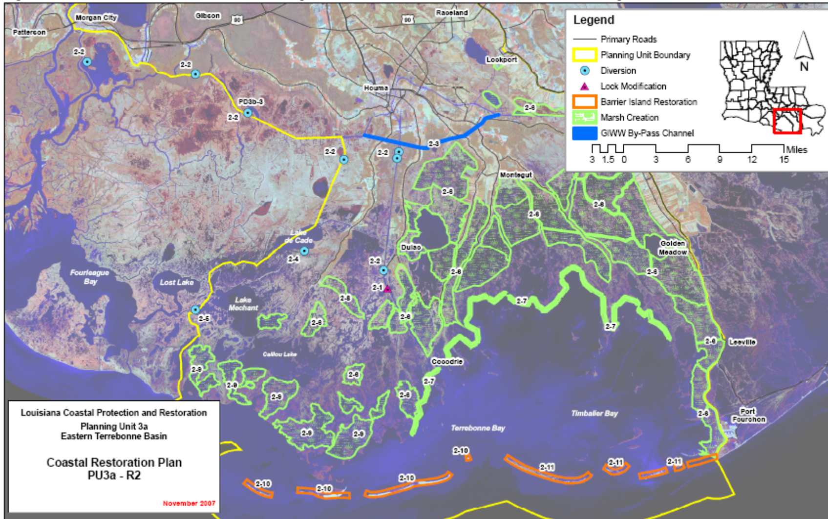
Figure 4c. Identified are the measures that comprise Alternative R2, GIWW Diversions – Planning Unit 3a.
