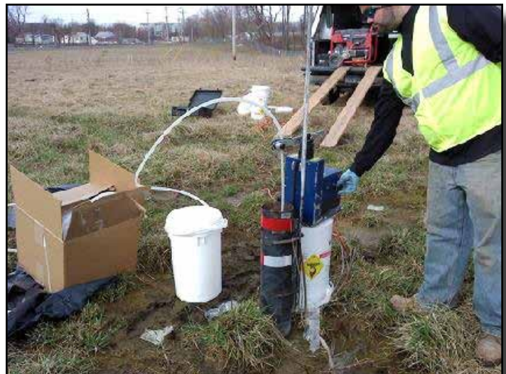
Sampling a groundwater well at the Colonie Site
