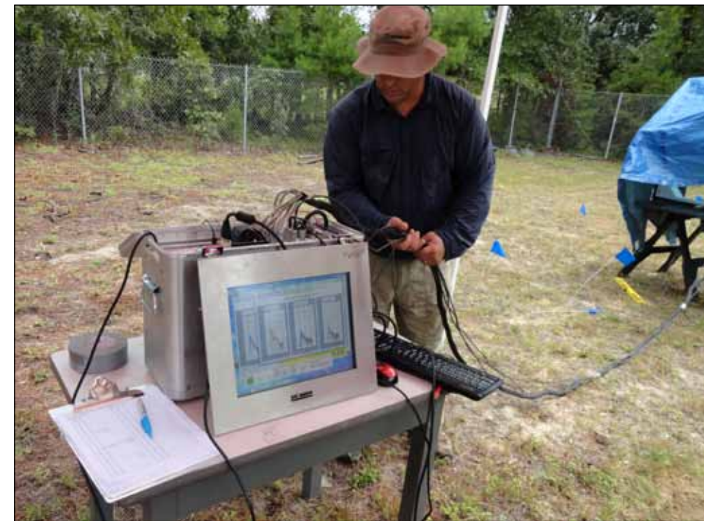
Andrew Schwartz connects cables to the MetalMapper system used to catalog munitions. The data will be used later at remediation sites. (Courtesy photo.)
