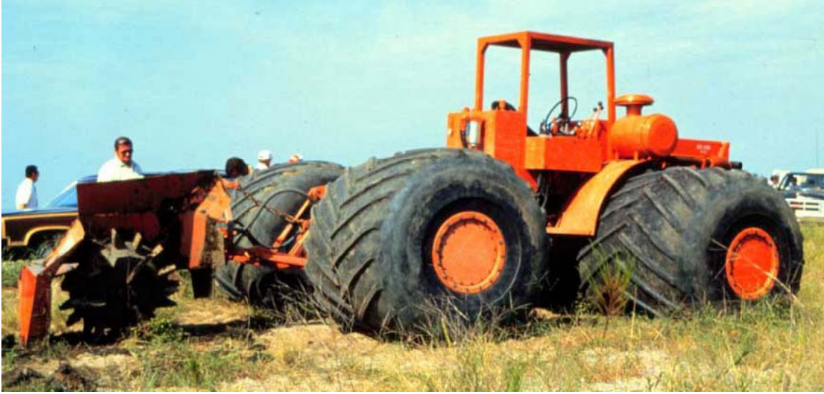
Figure 11. Rubber-tired rotary trencher
