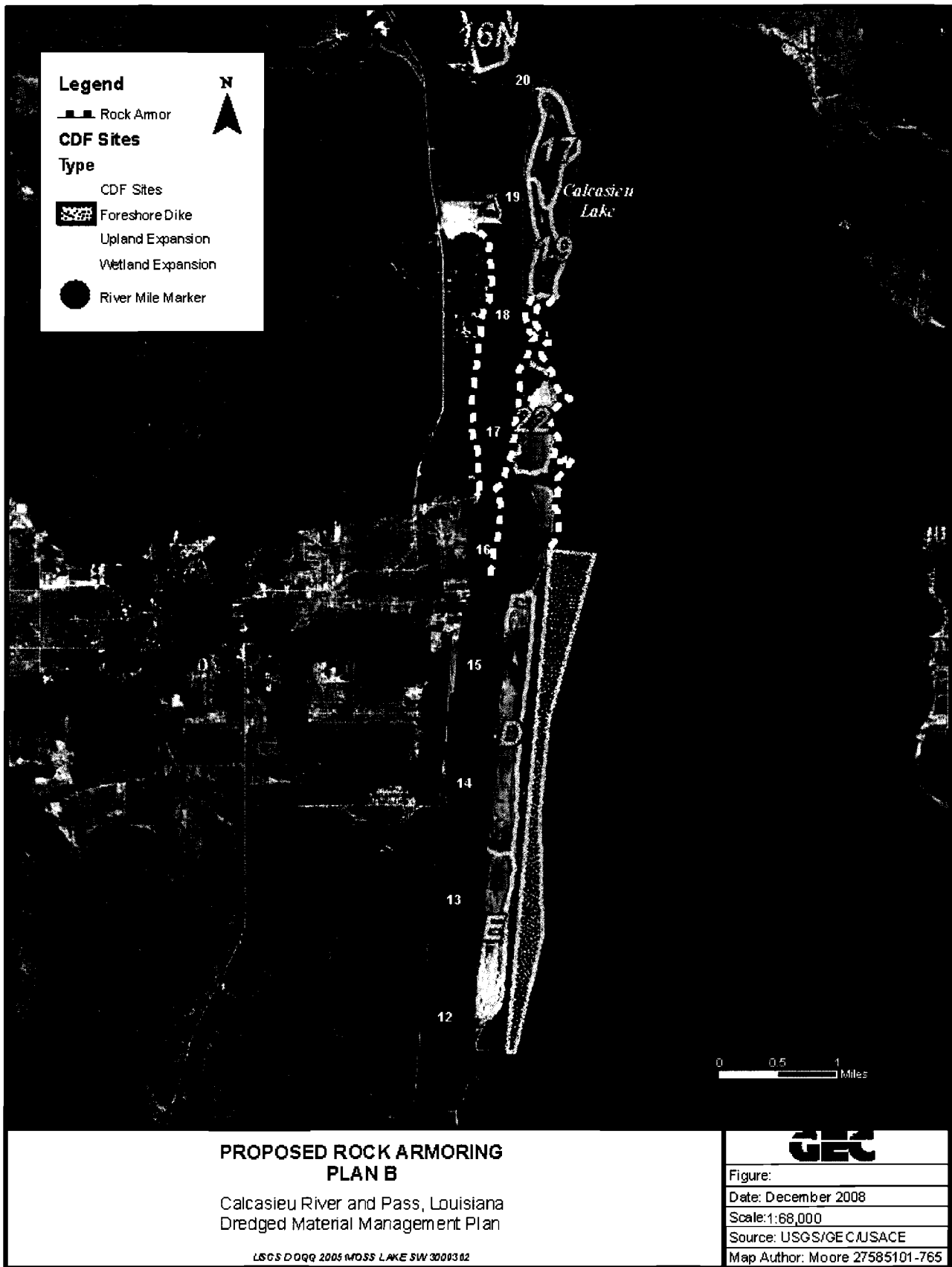
Figure 2. CDF and rock placement sites.
