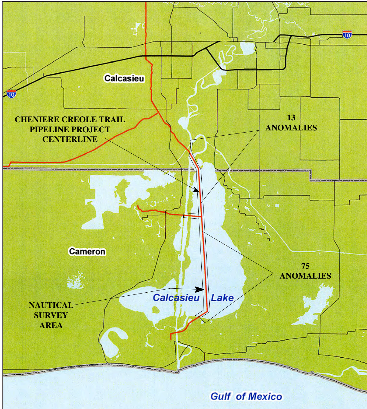
Figure 6-2. Cheniere Creole Trail Pipeline Project corridor across Calcasieu Lake (Enright et al. 2005:3). Note that 88 magnetic anomalies were detected along this corridor, 75 in the southern portion and 13 in the northernmost portion. All are interpreted as potential historic shipwrecks.
