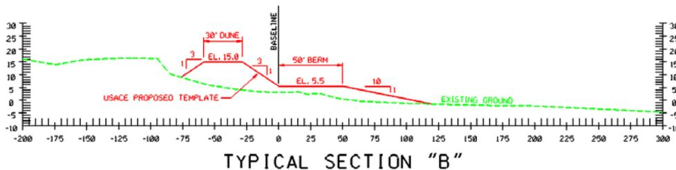
The recommended plan includes the initial fill and four renourishments, for a total of five nourishments, in 50 years at an average of 10-year intervals. Initial construction of the recommended plan will require the placement of 3,868,000 cy of material and a total of 7,157,000 cy for the four renourishments which average 1,789,000 cy of material each cycle. Other associated features of the project are dune
