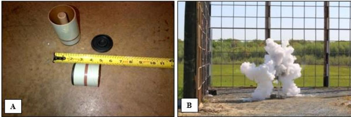
Figure 1. A) Explosive dissemination test item and B) explosive test item function with TiO<sub>2</sub> payload.
