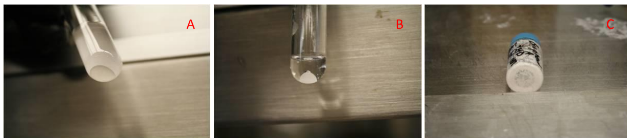
Figure 6. Products obtained by different processing methods. Product A reacted and received ice water to precipitate product; Product B reacted, received water to precipitate product, and reacted for three additional hours; and Product C formed product immediately, used NaOH prepared in water and received no additional heat or mixing.
