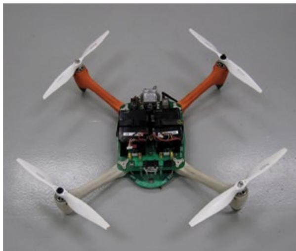
ECBC used its rapid engineering design and additive manufacturing (3-D printing) capabilities to fabricate the unmanned aircraft system.
