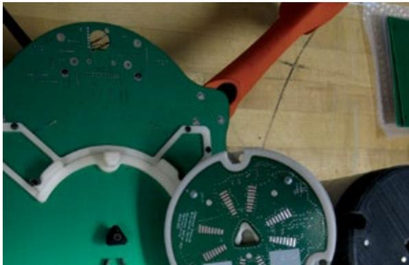
ECBC’s Unmanned Systems Team researched and evaluated commercial off-the-shelf (COTS) unmanned aircraft systems, and then made its own version, including the innovation of using a circuit board to act as the structural frame.
