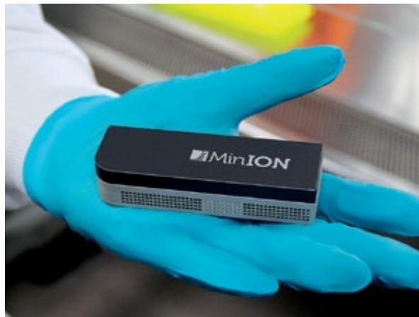
ECBC is working with a revolutionary new DNA sequencer, known as the MinION™ which fits into the palm of the hand and is perfect for use in remote locations to characterize strains of viruses and bacteria by determining their genetic fingerprint.
