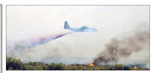
Air Guard crews flying C-130s equipped with Modular Airborne Firefighting Systems (MAFFS) flew 367 sorties and dropped more than 880,000 gallons of fire retardant on wildfires in the western U.S. in FY13, lessening the risk to firefighters and civilians while protecting critical infrastructure and personal property.
