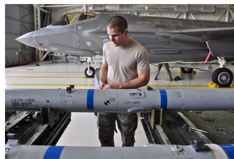
AMRAAM A1C Zoller makes an AIM-120 advanced medium-range air-to-air missile safe before loading it onto an F-35A Lightning II.
