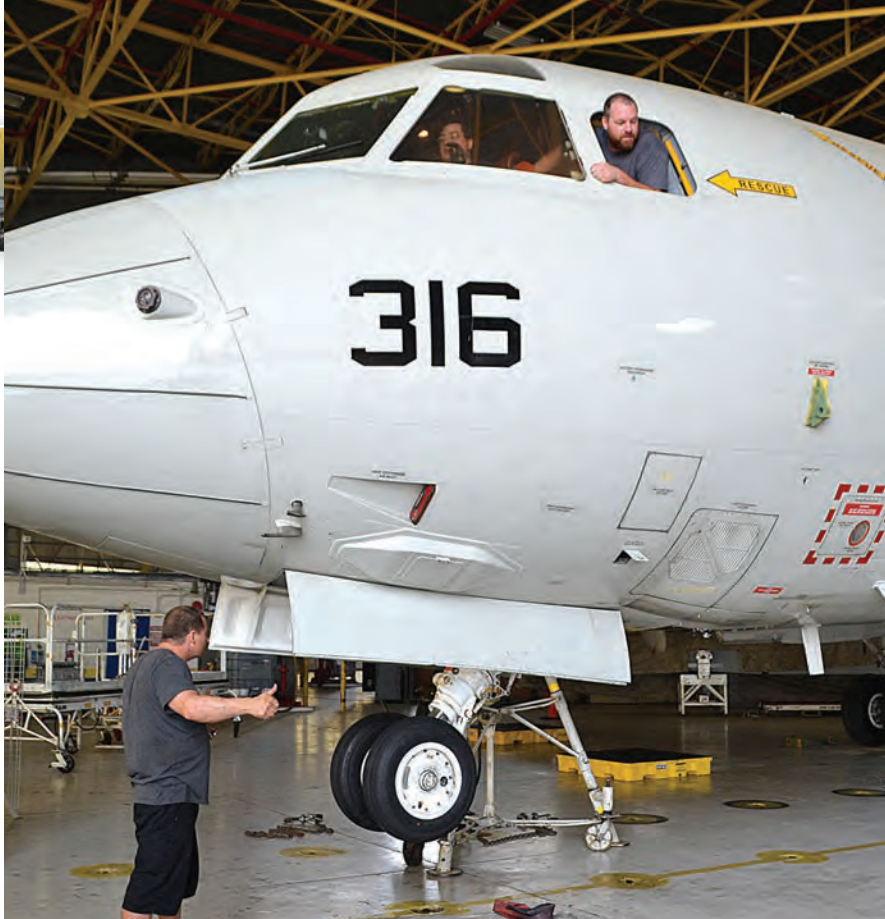
Artisans at Fleet Readiness Center Southeast (FRCSE) in Jacksonville, Fla., test the functionality of a P-3 Orion's landing gear. A team of tool designers, artisans and engineers from FRCSE used additive manufacturing to repair the Orion's wheel-well truss.
