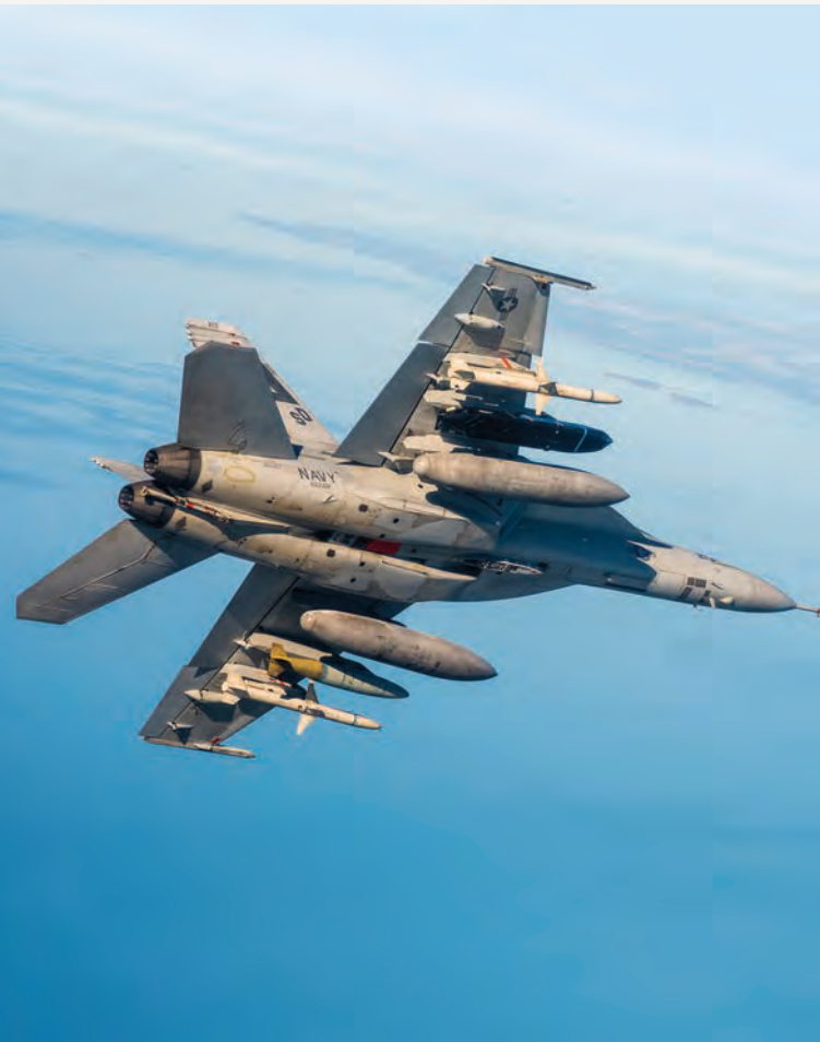
An F/A-18 carries a model of the Long Range Anti-Ship Missile (LRASM) during a flight test over Patuxent River, Md., completing the first phase of inflight loads testing for the weapon program.
