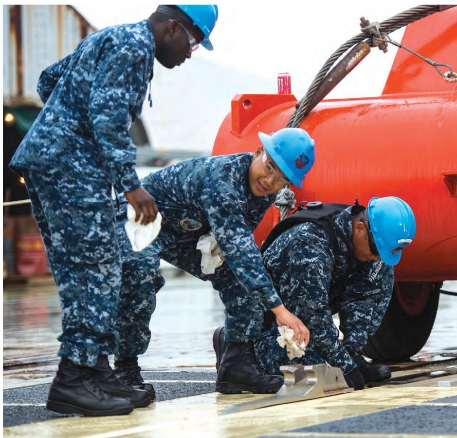
Sailors from PCU USS Gerald R. Ford (CVN 78) prepare to launch a dead-load sled from the ship's Electromagnetic Aircraft Launch System (EMALS).
