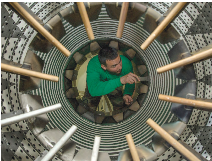
An aviation machinist's mate inspects an F/A-18 afterburner in the jet shop aboard Nimitz-class aircraft carrier USS George Washington (CVN 73).
