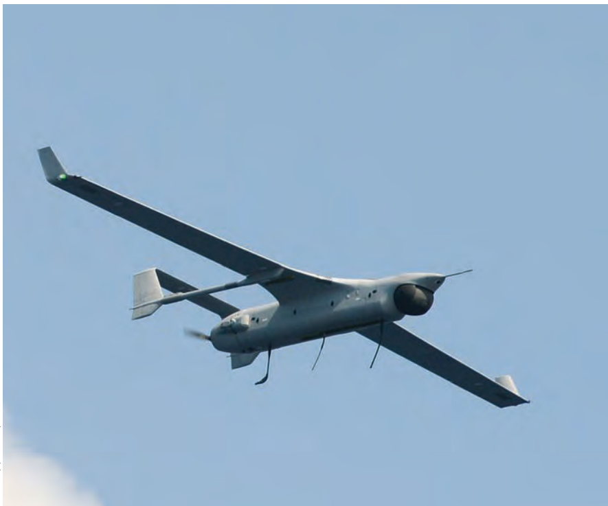
The unmanned RQ-21A Blackjack is a twin-boom, single-engine monoplane for surveillance and reconnaissance. It can be launched and recovered on land or at sea without runways, using a pneumatic launcher and net-type recovery system.
