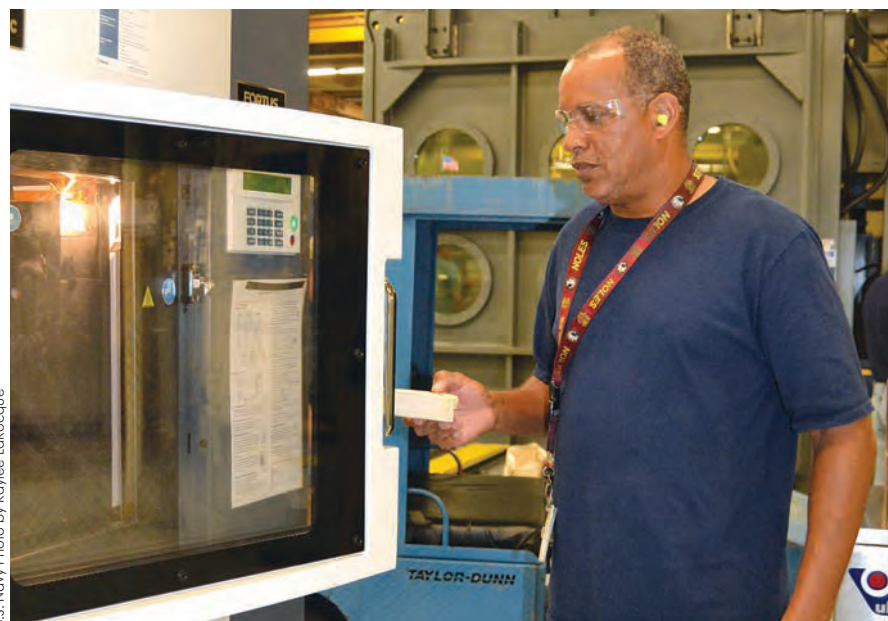
A Fleet Readiness Center Southeast sheet metal worker removes a modeled form block for an F/A-18 Hornet bracket from the Statasys Fortus 400mc printer in the military depot's manufacturing division. The printer creates the 3-D model from a computer-aided design one layer at a time using a thermoplastic product. The modeled form block is then used to form the metal bracket used on the aircraft.
