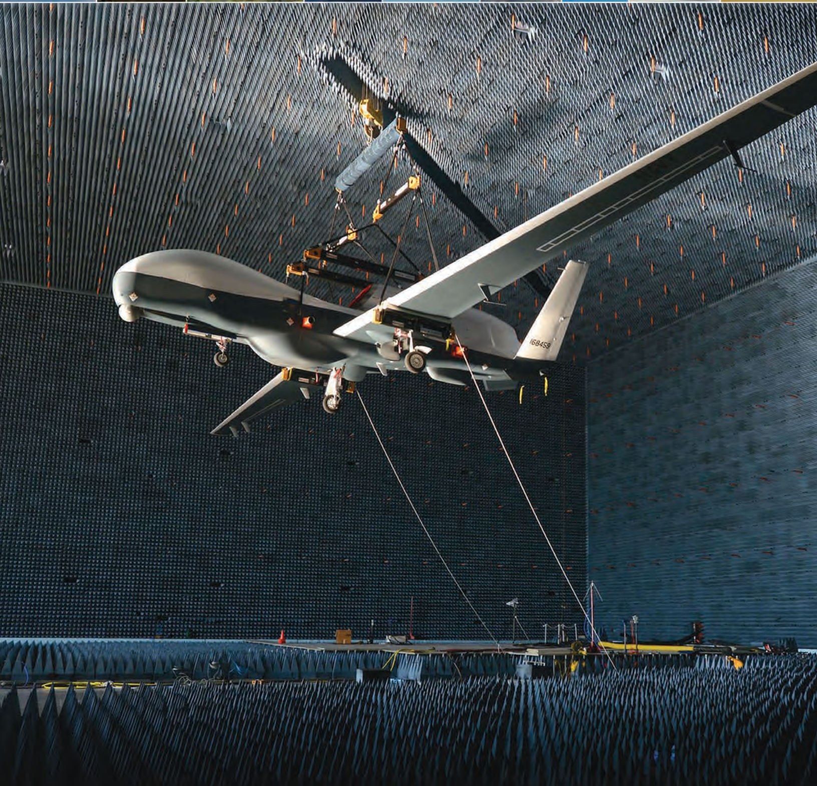
An MQ-4C Triton is lifted inside an anechoic chamber for electromagnetic compatibility testing at Patuxent River, Md. This event marked the first time that an unmanned aircraft inside the chamber was controlled from an external ground control station.
