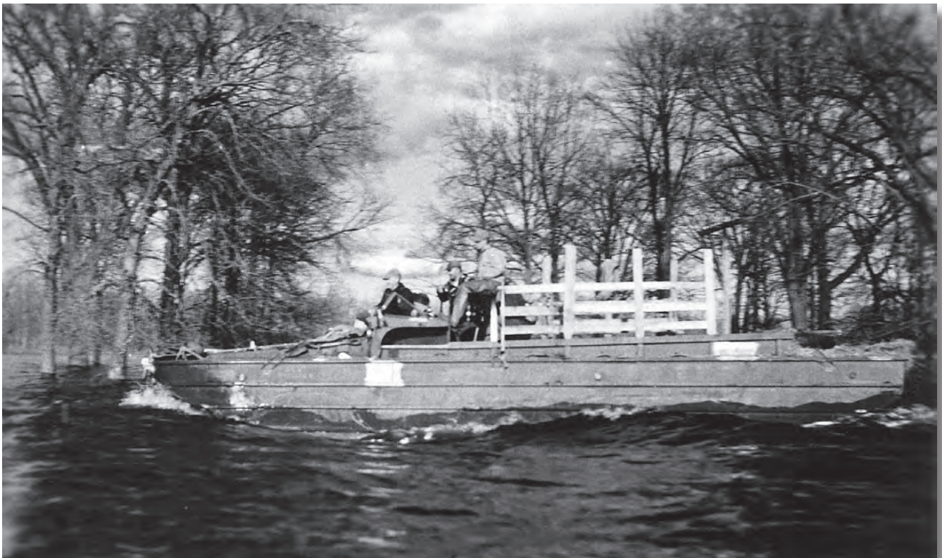
Engineer soldiers patrolled near Aitkin, Minnesota, in an amphibious DUKW. The vehicle was equipped with a makeshift rack in case of livestock rescue.
