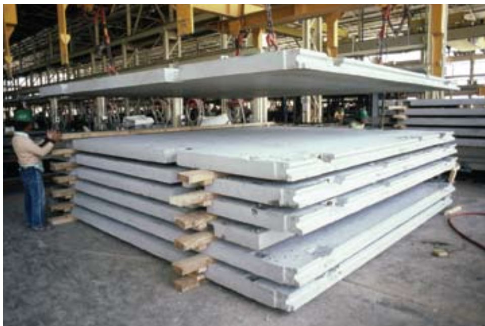
Precast concrete stacked for storage at Hafar al Batin
