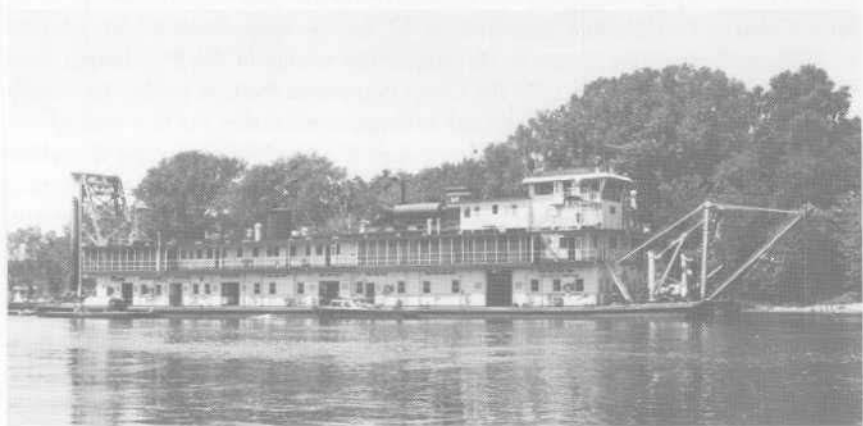
The dredge William A. Thompson , 1968. Boats such as this dig or pump out material from the river bottom to deepen the channel.
