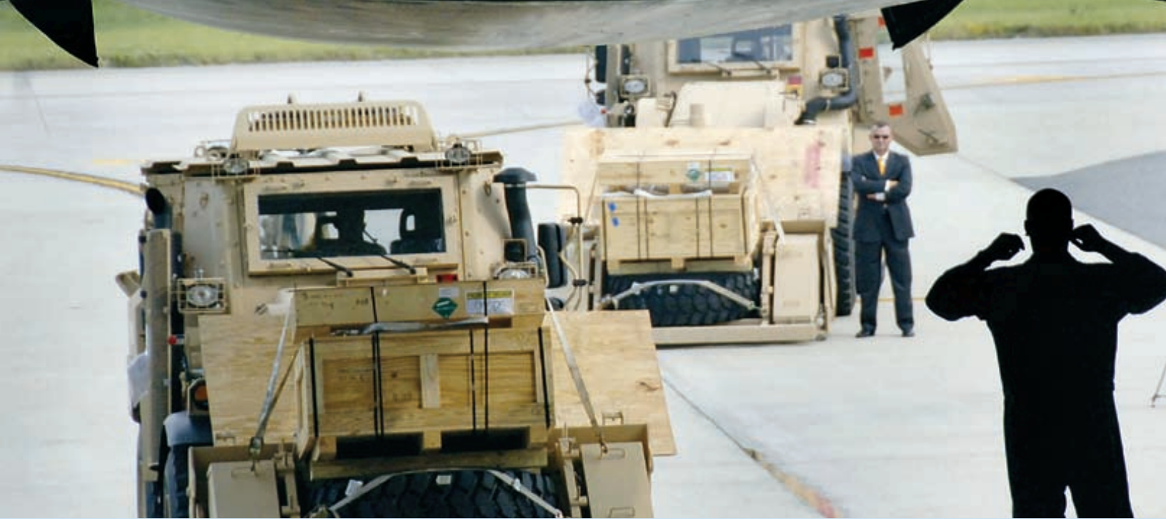
A Tennessee Air Guardmember guides an Army high-mobility engineer excavator into the back of a C-5 Galaxy.
