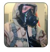
to simulate exposure to chemical agents, volunteers don test items and enter a test chamber containing a polydispersed corn oil aerosol challenge. The corn oil aerosol is between 0.4 and 0.6 micron in diameter and has an air concentration of 20-40 mg/m3. The air inside the protective equipment is
