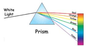
A prism is a specially shaped crystal. When white light shines through a prism, the light is separated into all its colors.
