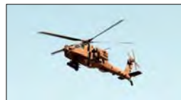
1. An AB3 with no mast-mounted assembly (Slick)
