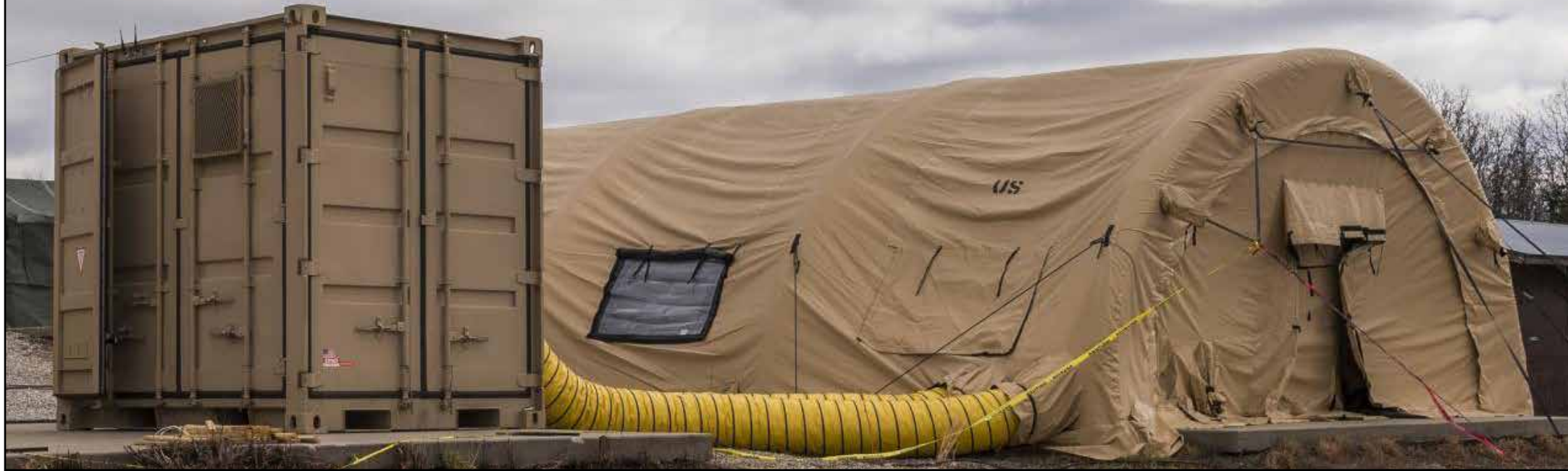
Natick's Minimized Logistics Habitat Unit, or MILHUT, is a containerized shelter that relies on renewable energy technologies that enable warfighters to be deployed longer in remote areas without the need for resupply. (Photo by Jose A. Miletti, NSRDEC)
