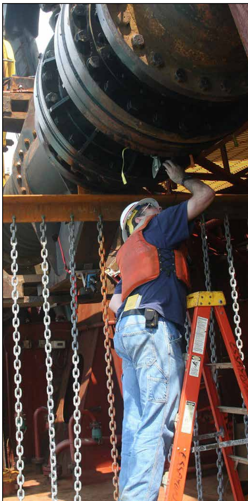
ABOVE: ERDC Research Hydraulic Engineer Tim Welp installs a GoPro camera to capture movements of the tickler chains designed to move sea turtles out of the way of dredging activities. TOP RIGHT: The chains form a curtain extending off the dredging drag arm approximately 25 feet ahead of the draghead. RIGHT: Sonogram monitoring of tickler chains designed to move sea turtles away from dredging areas. Clockwise from right are Stephen Willis, San Francisco District, Dena Dickerson, ERDC research biologist, and Tim Welp, ERDC research hydraulic engineer. (Photos by Jon Hosaka, Hawaii District)
