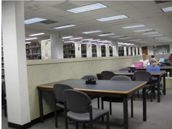
Half-height walls on column lines in several parts of the library are a clever way to offer access to power outlets in otherwise open areas with few walls.
