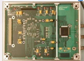
Digital Detector for RFI Detection (Ground Truth) IIP-04: Christopher Ruf
