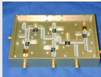
Controlled-Correlation Calibration Subsystem ACT-99: Ed Kim & Jeff Piepmeier
