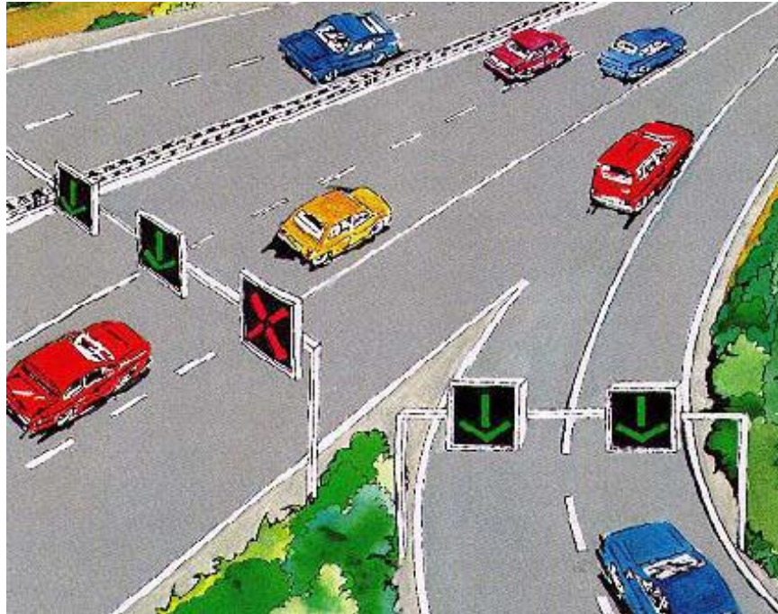
Figure 10. Dynamic Junction Control Schematic (Source: BASt, Germany).
