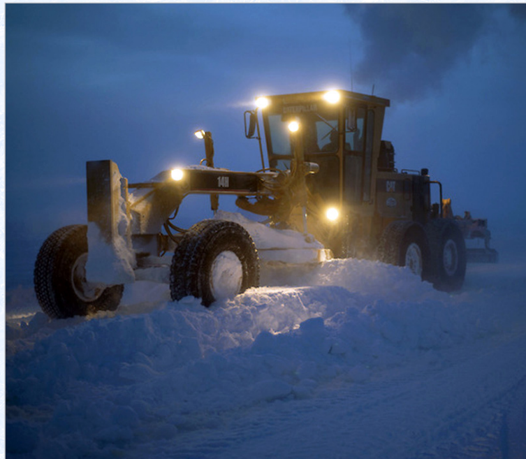
TxDOT uses a wide variety of heavy equipment during severe winter weather storms – including modified motor graders like the one pictured at left – to clear ice and snow from the roadway.
