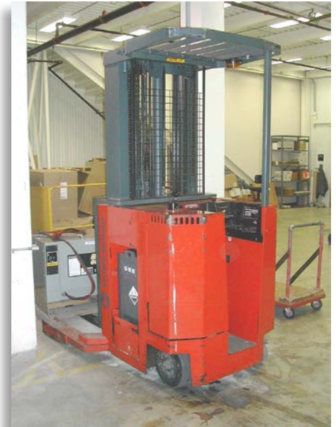
This Type E electric-powered industrial truck and the adjacent charging unit should be located and maintained to prevent fires.
