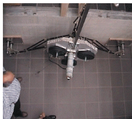
Landing Gear – three-legged device to secure safe landing as demonstrated here during tests at Lindau.
