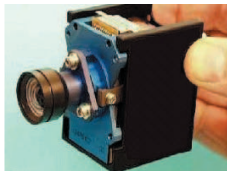
Photo 4: The CIVA micro-cameras-3D technology packaging, allowing to minimise volume (< 90 cm 3 for the head), mass (< 100 g) and power (< 2 W), has been used. Tests down to -150 deg, for storage, and -120 deg, for operation, have demonstrated outstanding thermal behaviour.
