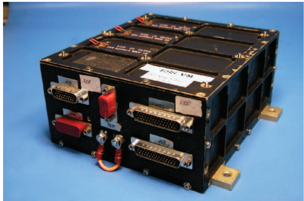
Electrical Support System (ESS) for the Philae Lander.
