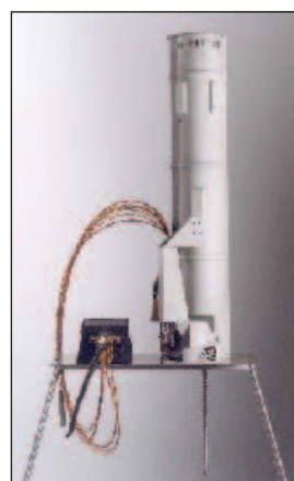
SD2: Sample Drill & Distribution instrument.
