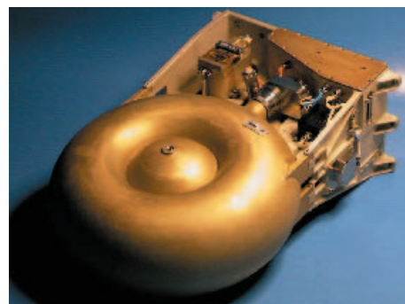
Active Descent System – cold gas system procured by DLR Cologne from Bleuler-Baumer, Oberrieden, Switzerland.
