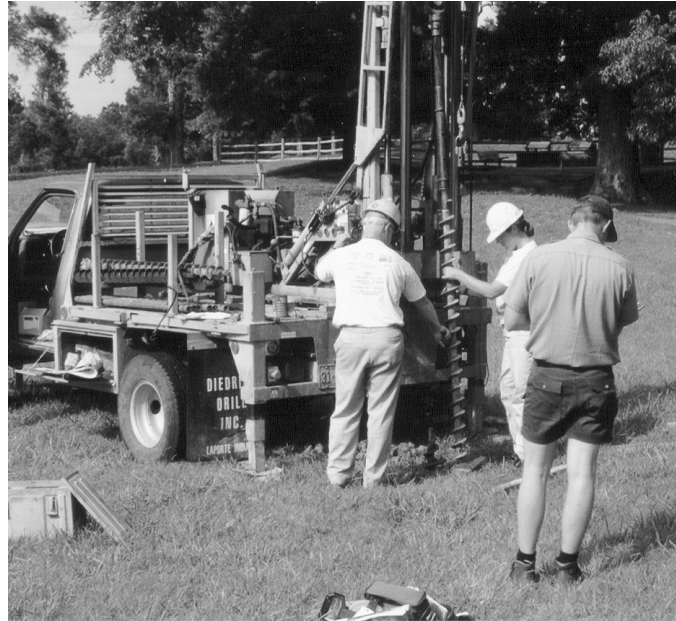
Dr. Bergquist and Petersburg National Battlefield personnel drilling a core hole at the Crater site. The tunnel lies below the area between the path and the drill.
