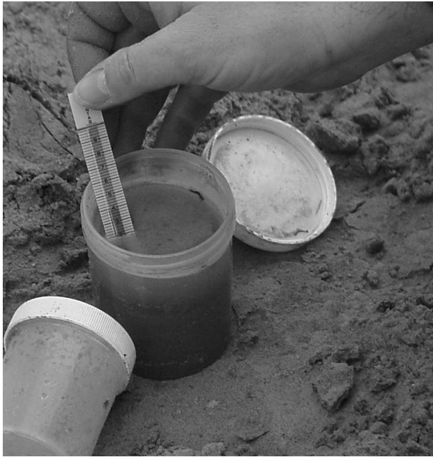
Chloride titration strips, used to measure salt in soil and water samples at oil and gas sites.
