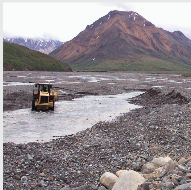
In-stream mining of sand and gravel along the Toklat River in Denali NP.
