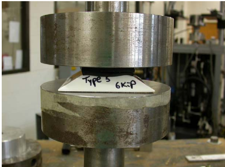
Figure 100. View of ASTM D 4280 Compression Test.
