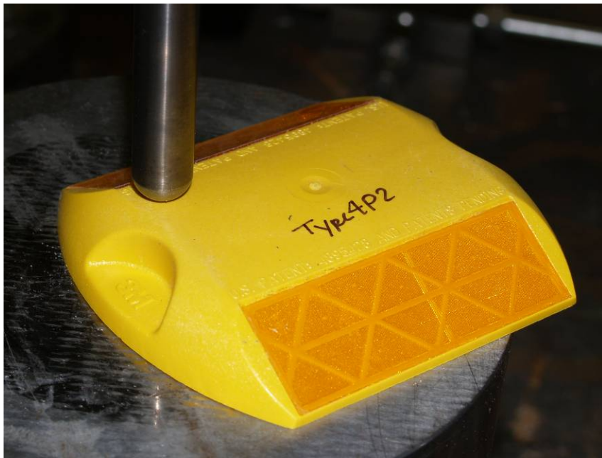
Figure 106. Poke Test with Rounded 1/2-Inch Diameter Rod.
