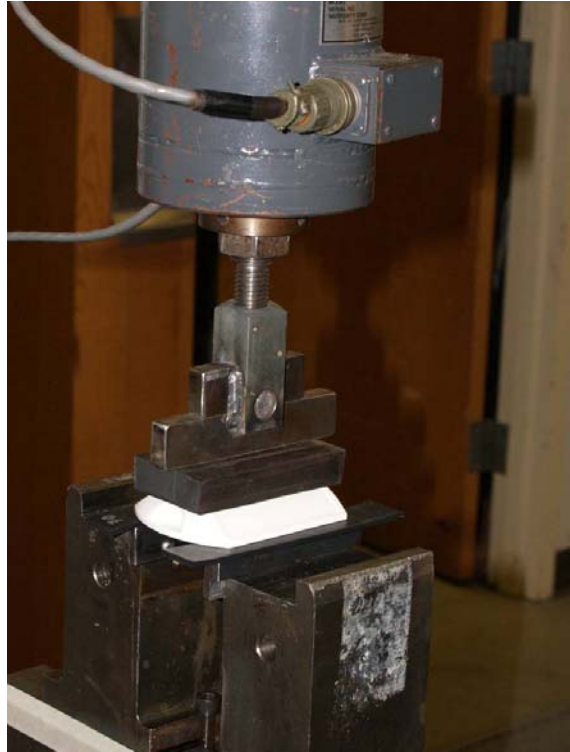
Figure 99. Test Setup for ASTM D 4280 Longitudinal Flexural Strength.
