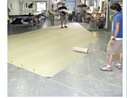
On the sail loft floor, a sailmaker lays out and cuts individual panels of sailcloth to a full-size template of the mizzen sail. These individual pieces of sailcloth are machine-sewn together to form the "membrane" of the sail.
