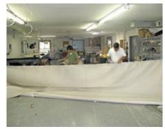
Sailmakers prepare for hand-sewing bolt rope around the perimeter of the spritsail. Bolt rope reinforces the edge of the sail and transfers wind energy to the rigging to drive the ship through the water.
