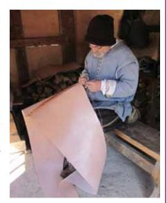
Historical interpreter Don Hulick sews a piece of leather in an early stage of the bellows construction project and tests the completed bellows.
