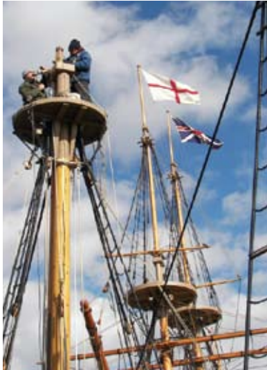
Marine mechanic Whit Perry and volunteer Rich Watkins prepare the topmast on Jamestown Settlement's Discovery for removal.
