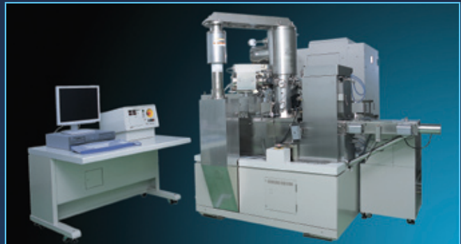
One of two electron beam lithography systems in the NanoFab. One resides in the class 100 cleanroom, the other in a high-performance laboratory outside the cleanroom.
