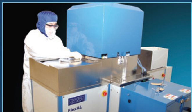
The NanoFab's atomic layer deposition system — one of five different deposition systems available — can deposit conformal, single atomic layers utilizing both thermal and plasma processes. The pictured system can deposit conformal layers of SiO 2 , Al 2 O 3 , HfO 2 , AlN, TiN and Ru.
