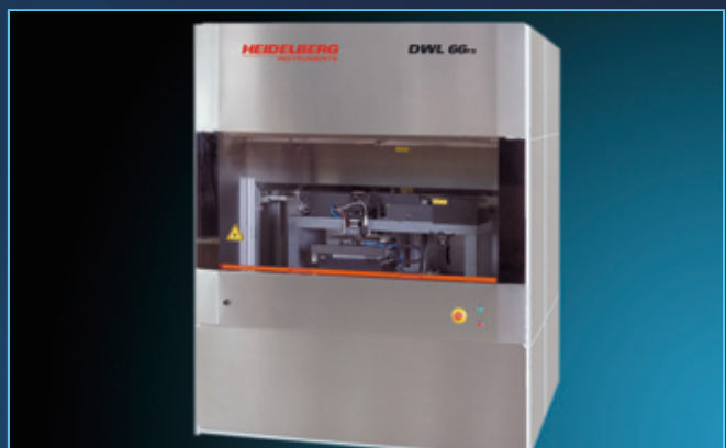
The NanoFab's lithography suite features a laser pattern generator targeted for low volume mask making and direct writing. The system can write directly to mask sizes from 25 mm x 25 mm to 150 mm x 150 mm, and to wafers from 50 mm to 200 mm in diameter.
