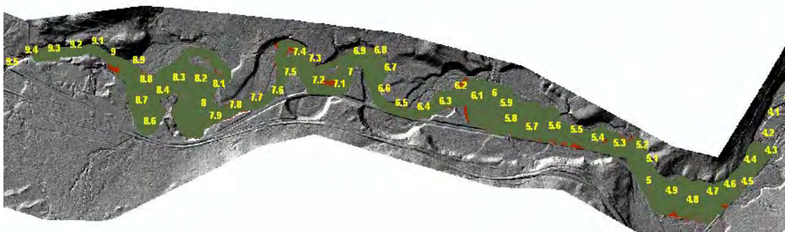
Figure 22. Inundation comparison of roughness of 0.04 (green) versus 0.05 (red) in geomorphic reach 1 for existing conditions. Areas in red represent the additional inundation caused by the higher roughness value in the active channel.
