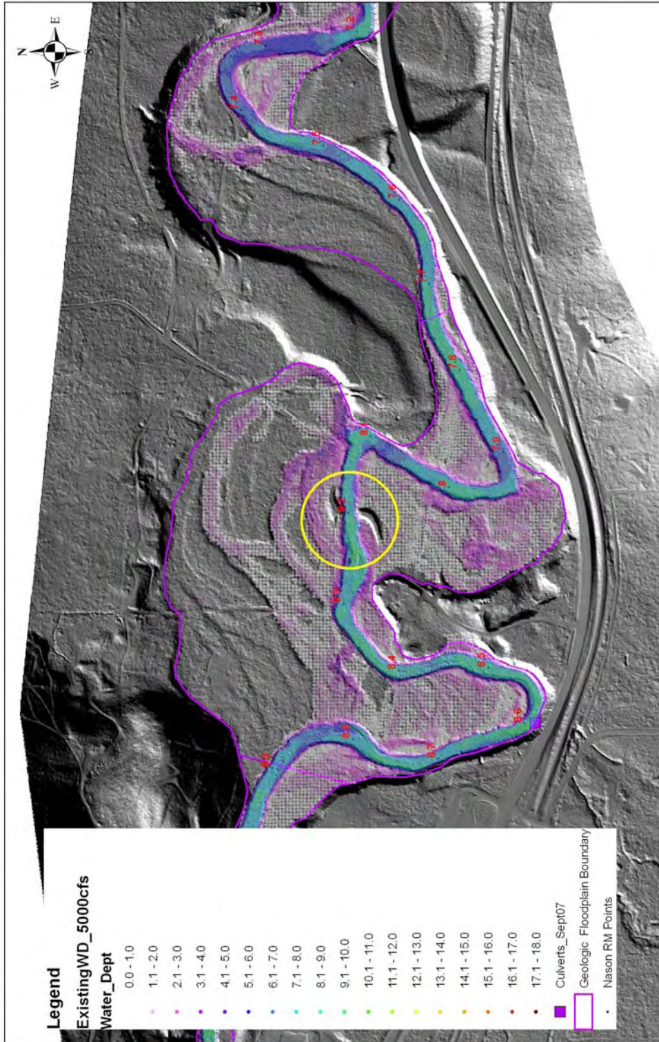
Figure 26. Impact to floodplain processes at RM 8 where flow can still go around embankment. Water depth (ft) results from the 2D model at a discharge of 5,000 cfs are shown, and are fairly shallow beyond the banks of the active channel.
