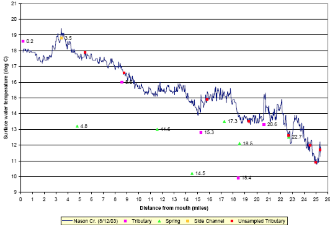
Figure 5. Median channel temperatures versus river mile for Nason Creek (August 12, 2003) (Watershed Sciences, LLC. 2003)
