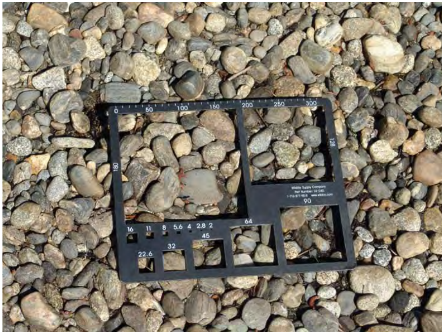
Photograph No. 9. View of gravel-sized material on a bar with gravelometer for scale. Kahler Reach; Subreach IZ-1, Nason Creek - Wenatchee Subbasin, Washington. Bureau of Reclamation Photograph by D. Bennett 8/9/07.
