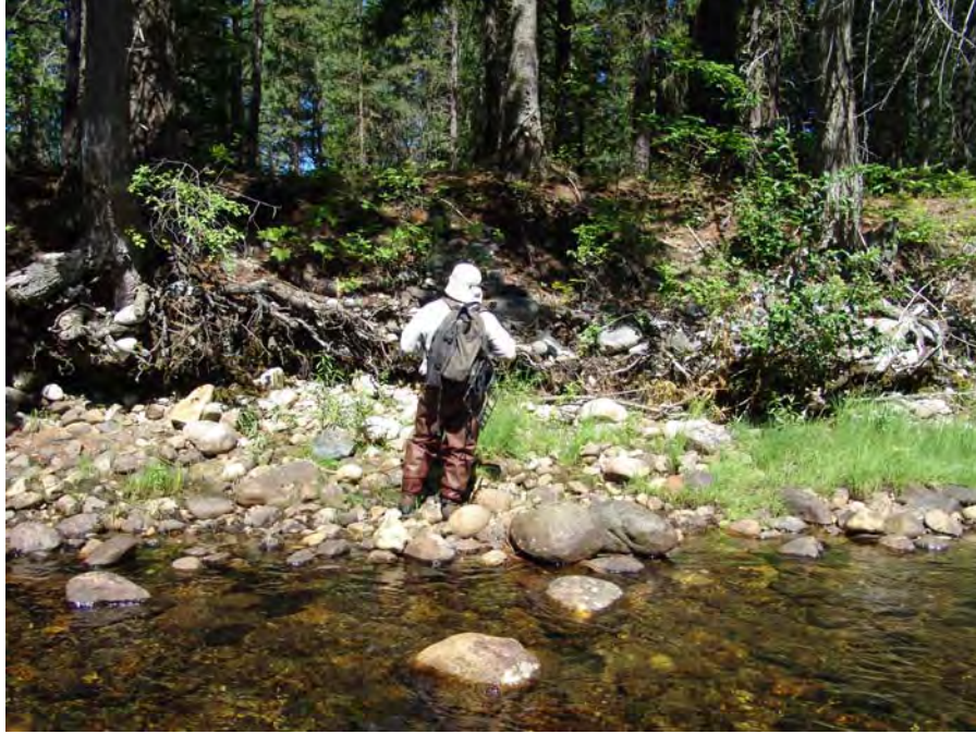
Photograph No. 12. View to the northwest showing cobble and boulder substrate and a 2 meter tall left bank. Kahler Reach; Subreach IZ-1, Nason Creek - Wenatchee Subbasin, Washington. Bureau of Reclamation Photograph by D. Bennett 8/9/07.
