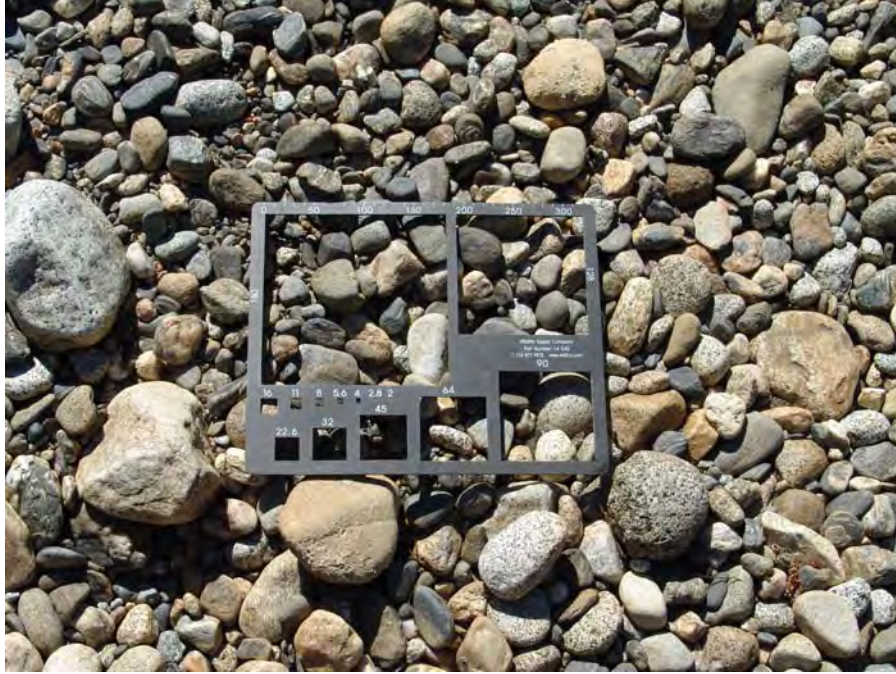
Photograph No.2. View of material located on bar with gravelometer for scale. Kahler Reach; Subreach IZ-1, Nason Creek - Wenatchee Subbasin, Washington. Bureau of Reclamation Photograph by D. Bennett 8/9/07.
