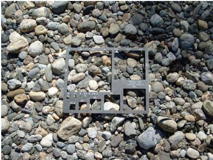
Photograph No. 15. View of gravel sized material on the bar with gravelometer for scale. Kahler Reach; Subreach IZ-1, Nason Creek - Wenatchee Subbasin, Washington. Bureau of Reclamation Photograph by D. Bennett 8/9/07.
