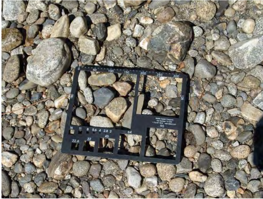
Photograph No.24. View of gravel and cobble sized material on a bar with gravelometer for scale. Kahler Reach; Subreach IZ-1, Nason Creek - Wenatchee Subbasin, Washington. Bureau of Reclamation Photograph by D. Bennett 8/9/07.
