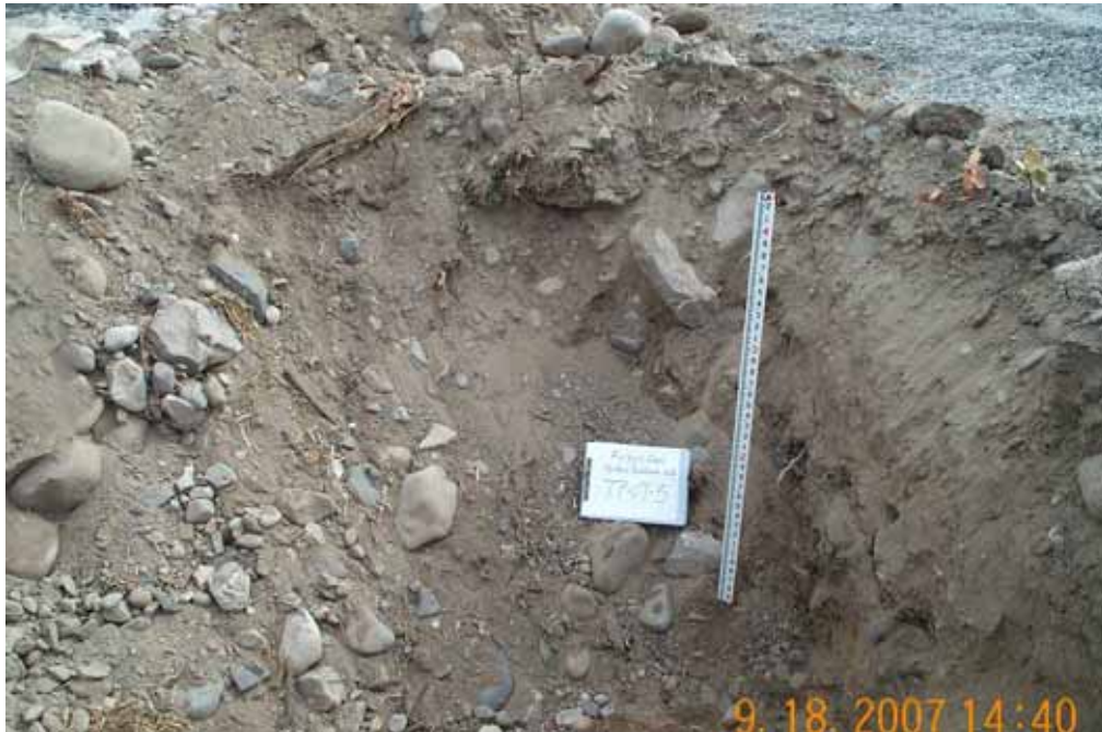
Photograph No. 15. View is to the south looking at test pit TP-07-5 excavated west of the riprap placed along the roughened channel on river right. Fulton Dam, Methow Subbasin, Washington – Bureau of Reclamation Photograph by E. Lyon, September 18, 2007.
