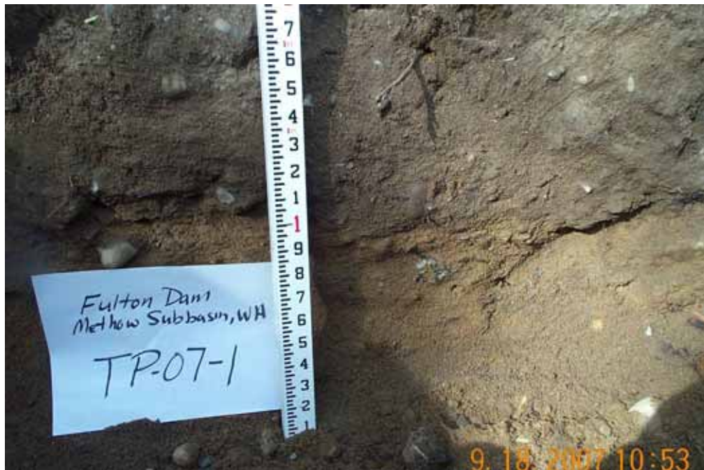
Photograph No. 11. View of spoil material overlying native or backfill material in test pit TP-07-1. Fulton Dam, Methow Subbasin, Washington – Bureau of Reclamation Photograph by E. Lyon, September 18, 2007.
