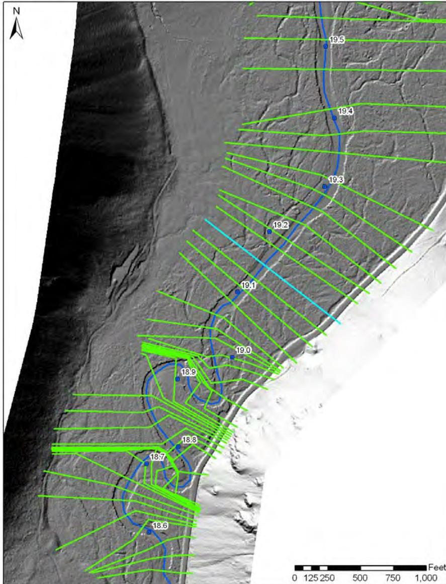
Figure 16. Example cross section spacing and alignment (highlighted cross section shown in Figure 17).
