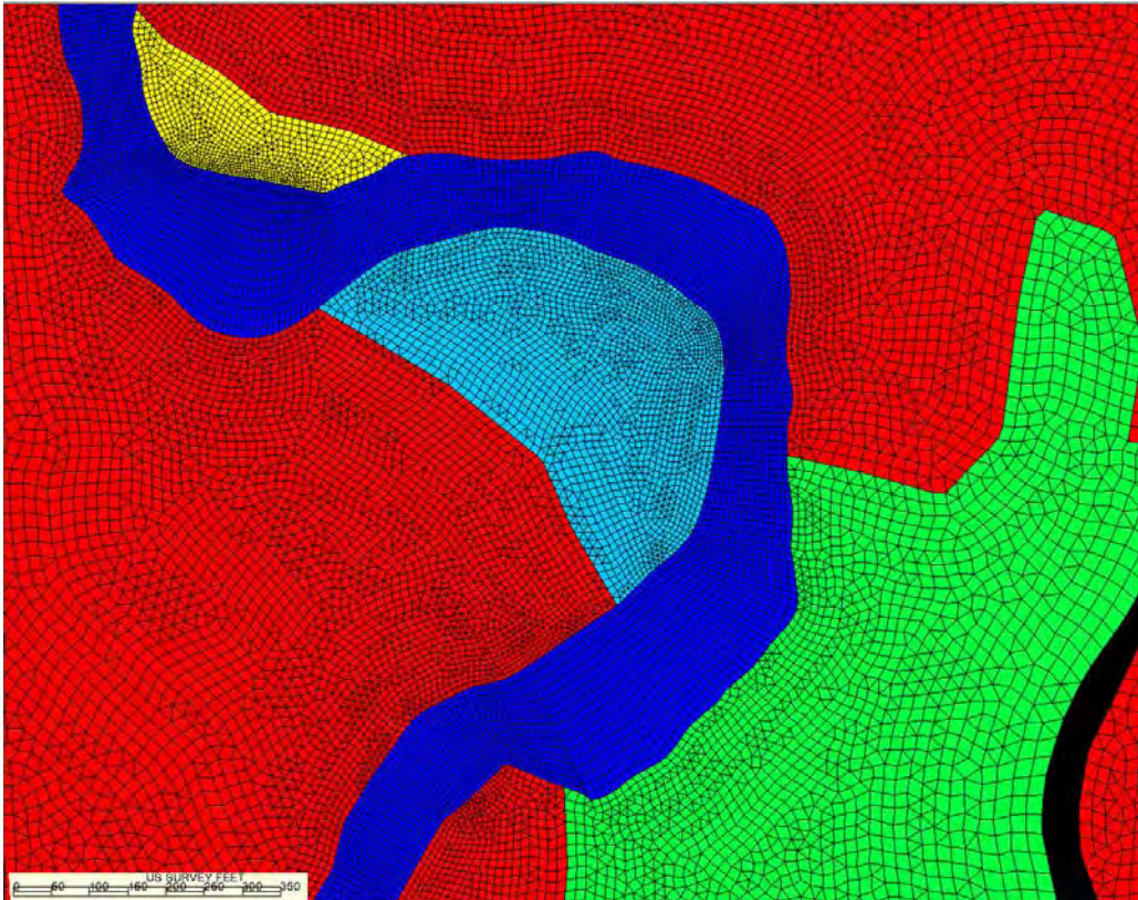
Figure 11. Example of model mesh in SMS. Colors represent various material types (dark blue = active channel, light blue = high flow bar, yellow = sparse vegetation, red = dense vegetation, green = cleared, black = road).
