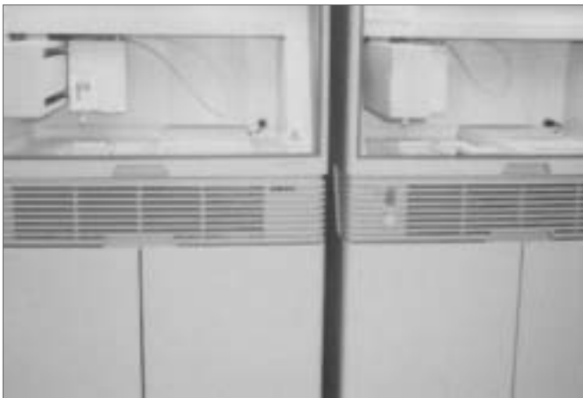
ABI 3700 Capillary Electrophoresis Units Sequencing Instruments used to determine the sequence of amino acids in DNA. (Photo Credit: Harvard Medical School/Partners Healthcare System for Genetics and Genomics and Biopolymers Facility Sequencing Core.)
