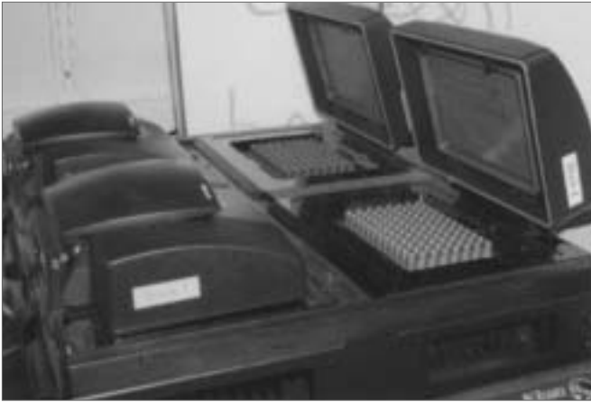
A Tetrad PCR Machine used for setting up polymerase chain reactions (PCR). The machine makes multiple copies of DNA from scarce genes. (Photo Credit: Harvard Medical School/Partners Healthcare System for Genetics and Genomics and Biopolymers Facility Sequencing Core.)
