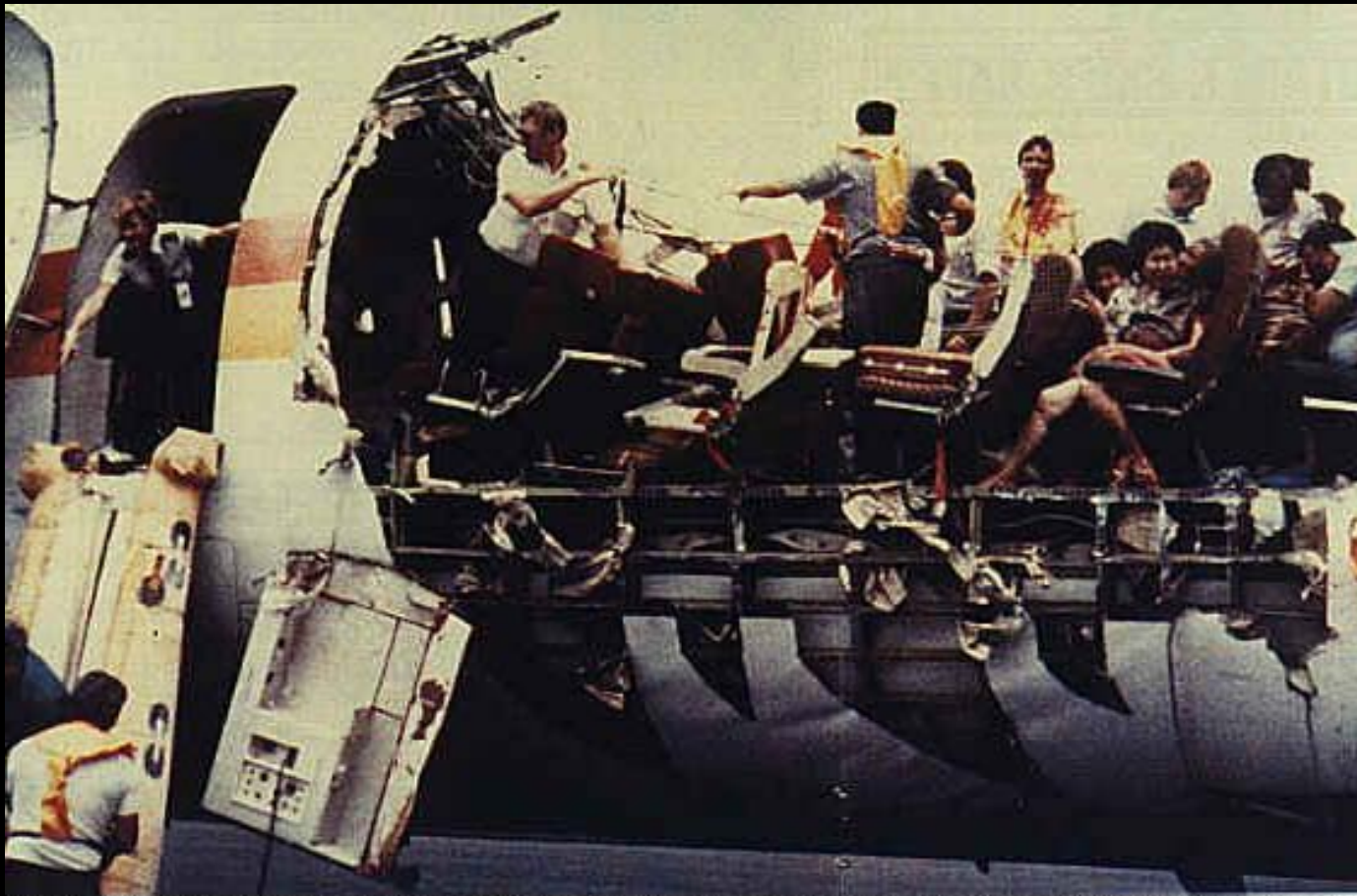
988 After 89,090 flight cycles on a 737-200, metal fatigue lets the top go in
