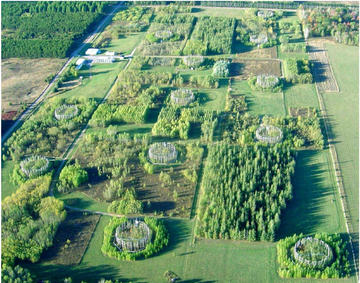
Figure 3. Infrastructure needs to study climate change impacts: FACE (Free Air CO 2 Enrichment) experiment conducted at Forest Service Northern Research Station facilities in Rhinelander Wisconsin. CO 2 is pumped out of pipes, controlled by sensitive anemometers, in order to assure a high CO 2 concentration at all times inside each ring. The photo shows several replicates of experimental (CO 2 , ozone) fumigations, and the control rings (no fumigations). FACE experiments require $1-$2 million in CO 2 supplies and maintenance yearly. Photo by David Karnowski, Michigan Technological University
